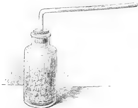
FIG. 3. Soaked Peas in Stopped Bottle, ready for Exhaustion of Air.
